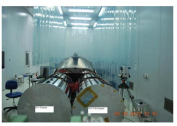
UVIT payload is to be launched on ASTROSAT and would make images in 28' field with a resolution < 2" in Far-UV (130-180 nm), Near-UV (200-300 nm), and Visible (320-550 nm). Testing and calibration of the two telescopes was completed. A photograph of the two telescopes shown above.
